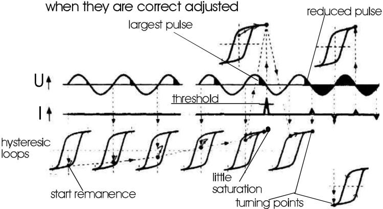
magnetizing wil be transported by the voltagetime-area pulses in the iron core.
